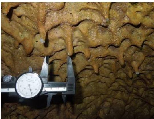
Fig.17 Lava stalactite of ChuBluck Volcano of Vietnam, C0Cave: P=3\sim 4\text{cm} , \gamma=560\sim 990\text{ dyne/cm}
