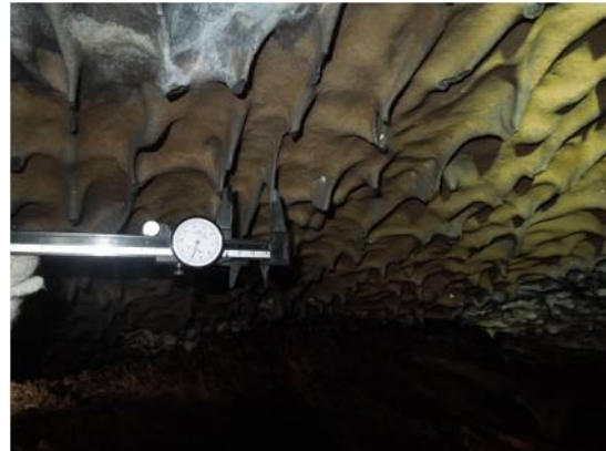
Fig.13 Lava stalactite on the ceiling of Mushpot Cave in Lava Bed National Monument: P=3\sim 4\text{cm}, \gamma=560\sim 990\text{ dyne/cm}
